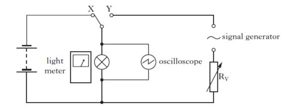
The switch is connected to X and the voltage across the lamp is  $2 \cdot 30 \, \text{V}$ . The reading on the light meter is recorded.
