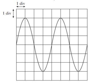
The time-base is set at 0.01 s/div and the Y-gain is set at 4.0 V/div.
