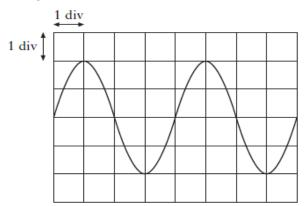
The timebase is set at 5 ms/div and the Y-gain is set at 10 V/div.
